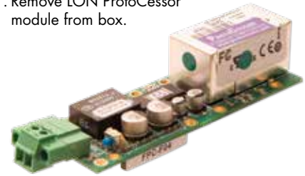
FIGURE 68-1: LON PROTOCESSOR MODULE INSTALLATION
