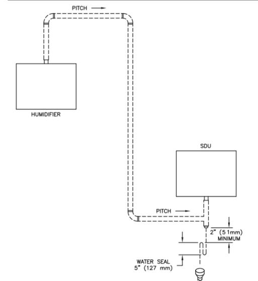
**FIGURE 2-2: SDU-E DRAIN LINE PIPING**
