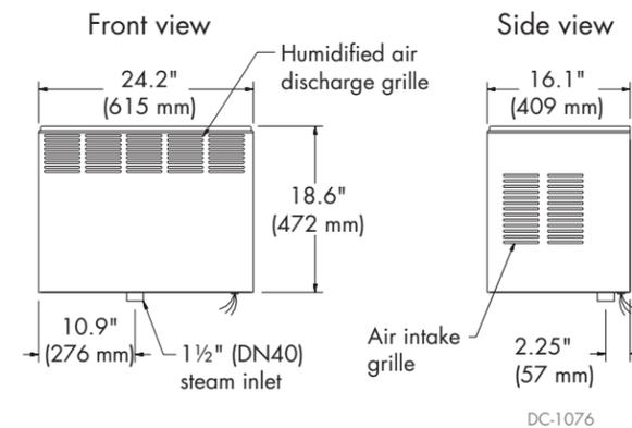
**FIGURE 1-2: SDU-E MECHANICAL DETAIL**
