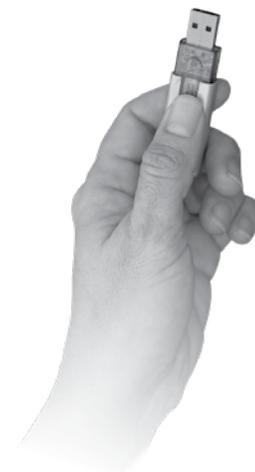
*Insert a USB flash drive into the Vapor-logic board's USB port to perform software updates, download data logs, and back up and restore data.*
